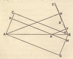
Huygens' principle the secondary wave from  $\mathcal{A}$  is at the instant t a sphere RNS of radius equal to  $\mathcal{A}G$ : the disturbance from H, after meeting the interface at K, will generate a secondary wave TV of radius equal to KM, and similarly the secondary wave corresponding to any other element of the original wave-
