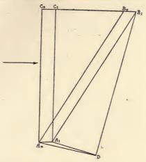
that light from a star is incident normally on this face. The rays experience no refraction at incidence; and we have only to consider the effect produced by the second surface  $A_0B_0$ . Suppose that during an interval  $\tau$  of time the prism travels from the position  $A_0 C_0 B_0$  to the position  $A_1 C_1 B_1$ , while the luminous disturbance at  $C_0$  travels to  $B_1$ , and the luminous disturbance at  $A_0$  travels to D, so that  $B_1 D$  is the emergent wave-front.
