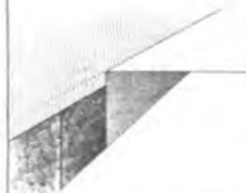
Enlarged perspective view of base of Granite walls Five Inches below Floor plate.
